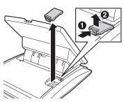
2. Plug the flat cable into the connector as shown.
